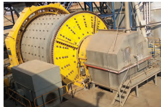
18' x 16' fully stainless steel mill for a milling-in-raftinate, copper application
